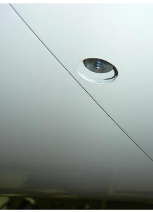
Secure the pin from upper side by the bolt – tightening moment is approx. 25 Nm.
