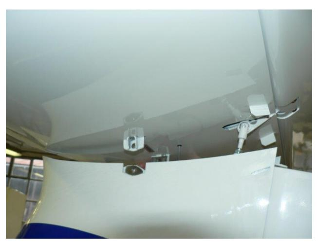
Connect the pushrod with the elevator control lever by the pin of  $\emptyset$  5mm and spacer + split pin. Connect the cable connector of the servo (in case of electrical trim option).
