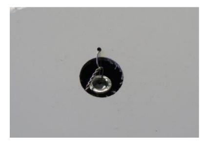
Finally, cover the hole on upper side of the HT with a white plastic sticker (to avoid water intrusion).
