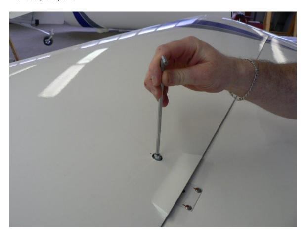
Come back to both main fitting screws M8 and tighten them fully.
